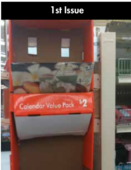
1st Issue No support at bottom of tray per shelf. Weight of product collapses the shelf bottom.
