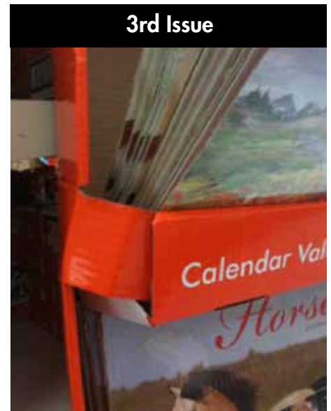
3rd Issue Quantity and weight of product in tray pushes shelf apart.
