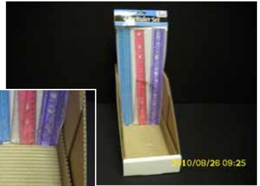
Use a wedge and single face corrugate material in bottom of PDQ tray to hold each item up-right and neat in PDQ.
