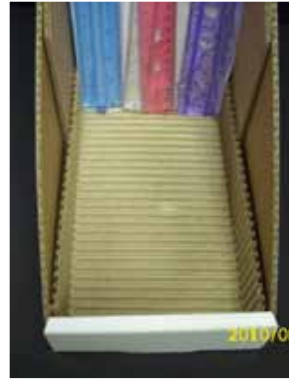
Use a wedge and single face corrugate material in bottom of PDQ tray to hold each item up-right and neat in PDQ.
